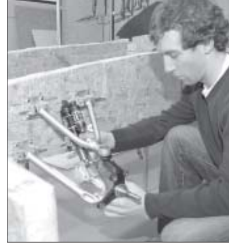
Walter Passarella/ News Advertiser photo Geoff Chadsey straightens out the Solar Vehicle prototype's wheel assembly.
