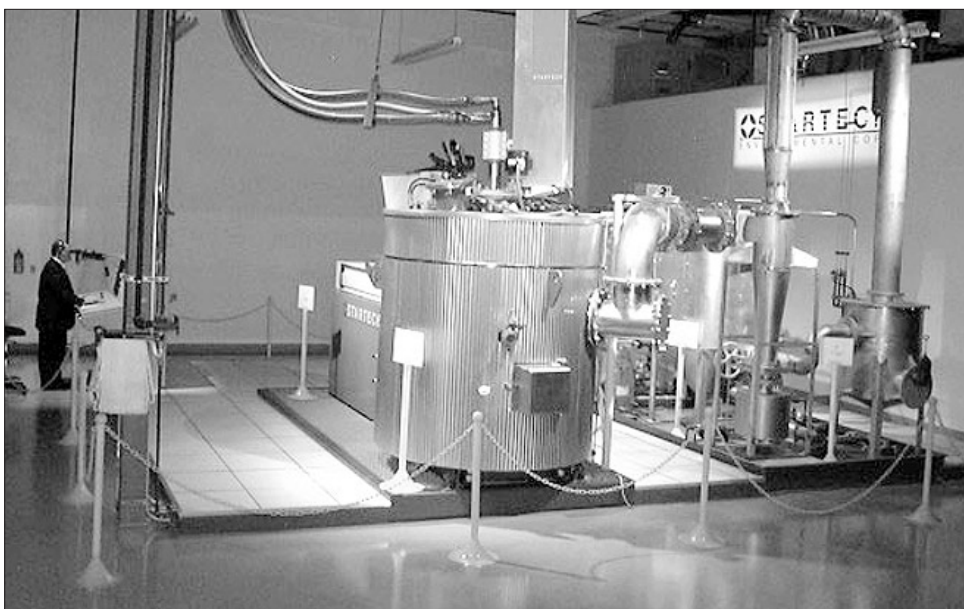
Ajax-based Pearl Earth Sciences Corporation is promoting the benefits of the Startech Plasma Converter, pictured above, which the company claims is the wave of the future in the waste management industry. Using a high-temperature plasma torch, waste is broken down to its elemental components.
